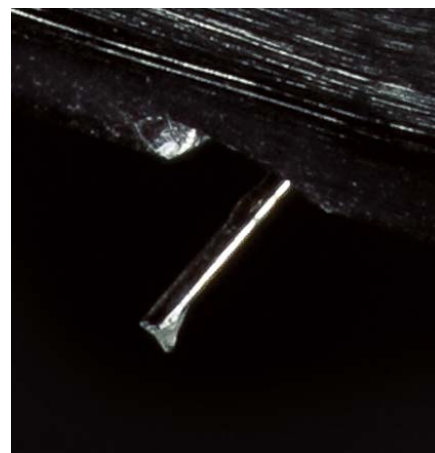
▲ Boron cantilever with a polished Shibata diamond stylus. Here are the convincing details.
