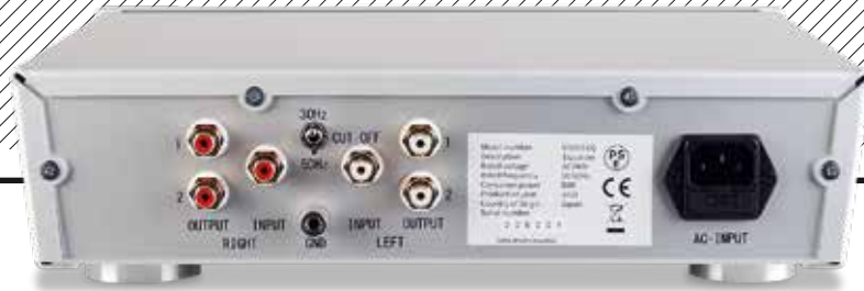
ABOVE: Rear view of the DS 003EQ PSU/equaliser. The pick-up's internal LED is powered via the R- and L- pins while the output is returned via R+ and L+, all via the 'Input' RCAs. The equalised outs are filtered at 30Hz or 50Hz (steeper via output 2)
