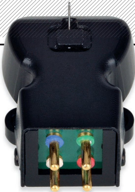
LEFT: Another view of DS Audio's precisely aligned boron cantilever and robust alloy body. The cartridge pins are gold-plated and well spaced to accommodate most tonearm leads/tags – power for the internal LED is supplied via the green and blue pins
